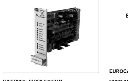
UEIK-2\* ELECTRONIC CONTROL UNIT FOR OPEN LOOP DOUBLE SOLENOID PROPORTIONAL VALVE SERIES 51
